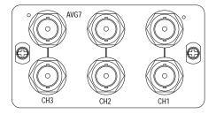
The AVG7 is an analog video generator for 525/625 interlace formats supporting component (Y'P'bP'r, R'G'B', Y/C), 525 Beta, and composite (PAL, NTSC, NTSC NoSetup). It provides two identical component outputs, two identical Y/C and Composite, or six identical composite outputs.
